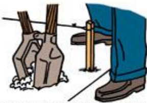
Space and dig the post holes every 6' to 8' apart.
