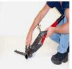
Wrap chain around pipe and engage nearest pin in upper jaw hooks.
