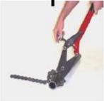
Rotate hand wheel clockwise to remove slack from chain.
